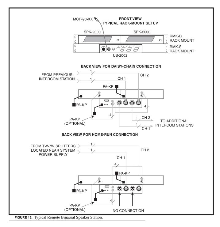
The configuration, shown in Figure 6, is similar to Figure 10, "Typical Remote Headset Station.," on page 21, except that each channel is heard in a separate speaker. Make sure the internal DIP switches are set for binaural speaker operation as described on "Monaural or Binaural Operation DIP Switches" on page 10. As in the previous example, a PA-KP local power supply is required for each SPK2000 speaker, but is optional for the US-2002.
