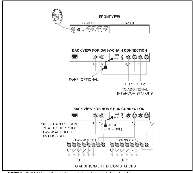
FIGURE 6. US-2002 Master Headset Station Configuration with 1 Power Supply.
