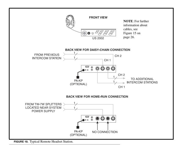
The configuration, shown in Figure 10, the US-2002 is not located near the system power supplies (SPS2001, PS2001L, etc.). The PA-KP local power supply is optional and can be used to power a single intercom station. When a PA-KP is connected to the US-2002, the US-2002 automatically disconnects from system power. This allows more system power for belt packs and other intercom stations. Also, when the US-2002 is powered by a PA-KP, it can be operated over a greater distance as a remote station.
